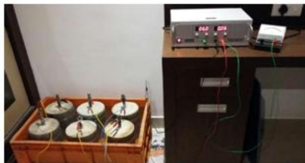
**Fig 2:** Impressed voltage test
